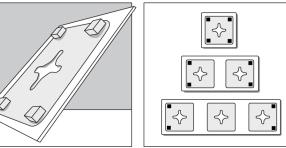
To the panels that span 1, 2 or 3 pegs, attach adhesive foam spacers to the back corners as shown above – on the paper.
