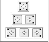
To the panels that span 1, 2 or 3 pegs, attach adhesive foam spacers to the back corners as shown above - on the paper.
